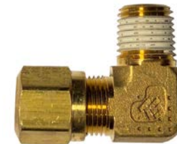
NY269-6-4 3/8T X 1/4P, NYLON TUBE, M ELBOW
