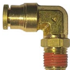
DOTS69-6-4 PUSH IN FITTING 3/8T X 1/4P, 90DEG, M ELBOW
