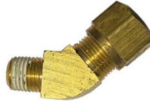
NY279-8-4 1/2T X 1/4P, NYLON TUBE, 45 DEG ELBOW
