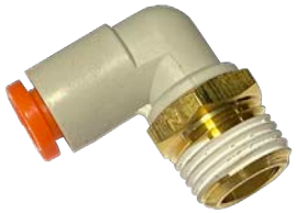
QL1369-3A COMPOSITE 90D ELBOW 3/16T X 1/8P
